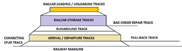
Figure 2 – Typical Ladder Track Terminal Configuration
