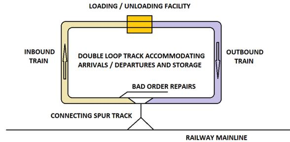
Figure 3 – Typical Loop Track Terminal Configuration
